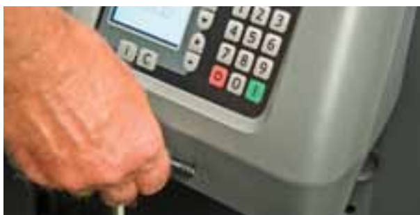
BT Optio H-series requires either a PIN-code or an ID key (option) to start
