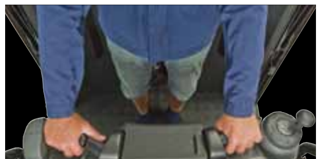
The multiple presence system ensures that the operator is safely in the cab before the truck can move
