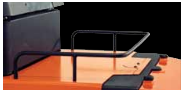
The OME100 and OME100W's parcel rail allows the top of the truck body to be used for temporary storage
