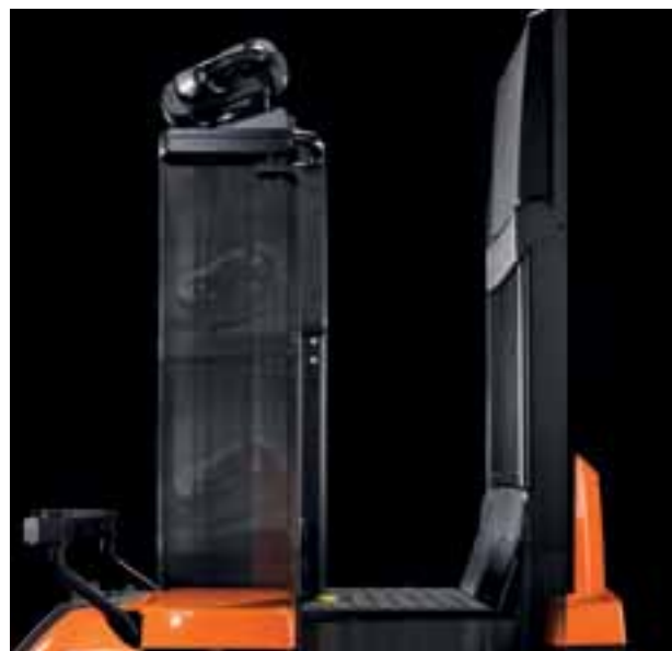
BT Optio L-series models with elevating platforms also have elevating controls, allowing manoeuvring and driving without having to lower the platform
