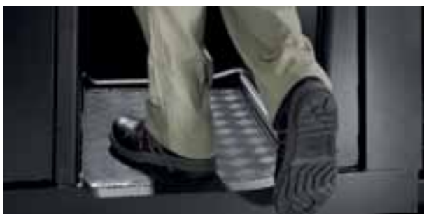
BT Optio's low step-in height reduces the strain of repeatedly stepping into and out of the truck. The floor is suspended to reduce vibration, helping some applications meet legislative requirements
