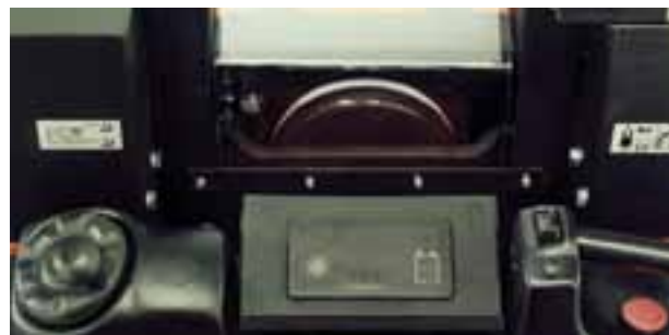
The comprehensive display shows lift height, battery status and drive-wheel position as well as warning and error codes
