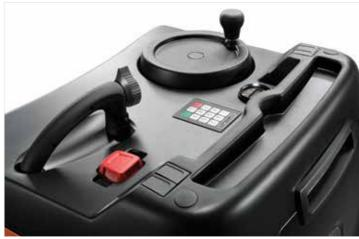
Spinner wheel' steering and PIN-code access
