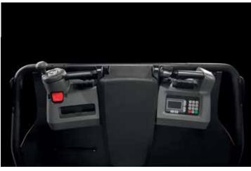
Ergonomic split controls are comfortable and improve access to the forks for picking
