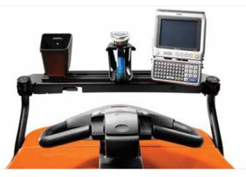
Optional powered E-bar allows easy mounting of ancillary equipment
