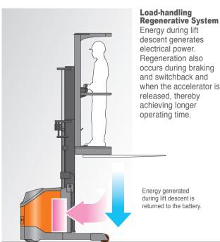
descent generates Regeneration also occurs during braking and switchback and when the accelerator is released, thereby
