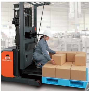
Together with a design emphasis on productivity for order-picking tasks, the low-height battery hood achieves a wide view to the front during travel.
